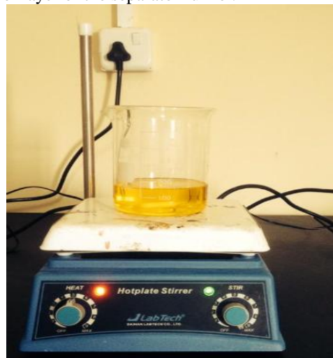
Figure 2: Hotplate Stirrer used in the optimization process.
